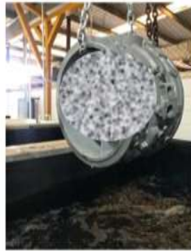
Scrap casting covered with grease and oil for the test
