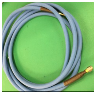
Figure 21 a 50 Ohms RF cable
