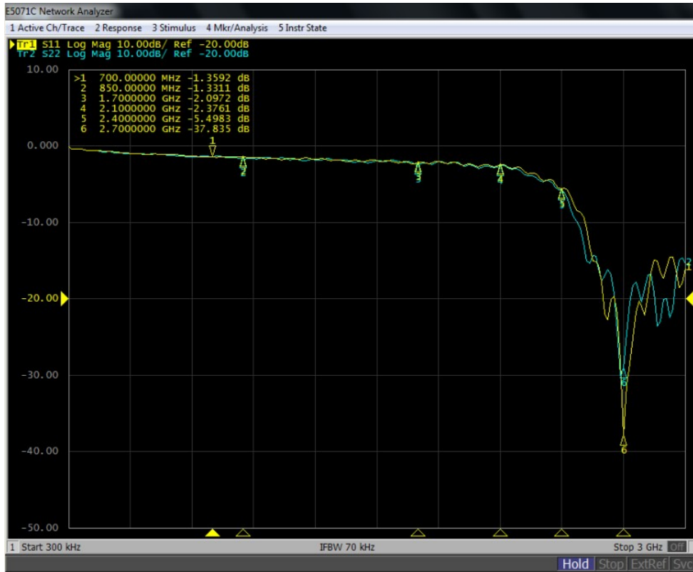
Figure 37 Site 1- S11and S2 - S22 scattering parameters measured at J5 HB HRM OUT point
