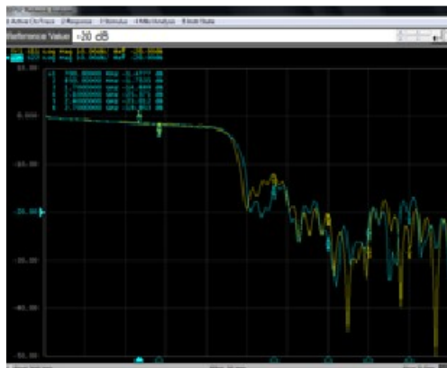
Figure 36 Site 1(S11) and Site 2 (S22) scattering parameters measured at J6 LB HRM OUT point
