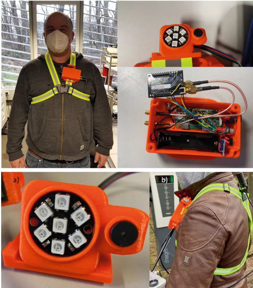
Fig. 4 Warning signal device. Source htw saar—ITS Research Group (FGVT)
